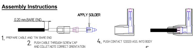
3. PUSH CABLE INTO CONTACT 103085 AND APPLY SOLDER TO CONTACT BUCKET
